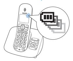
The battery icon displays the current battery level.
